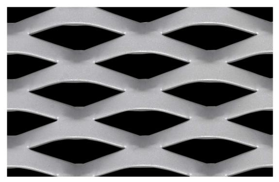
LW Pitch:76.00mmStrand Width:11.00mmSW Pitch:33.00mmThickness:3.00mmWeight:5.40 kg / m2Open Area:33%
